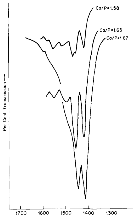
Fig. 1. Infrared spectra of hydroxyapatites of varying Ca/P ratios showing carbonate.
